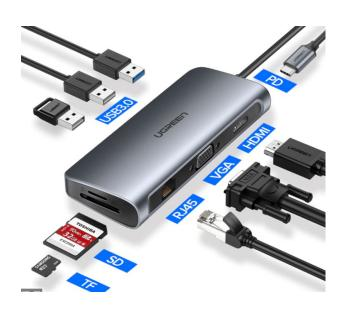
USB-C hubs (Also called USB-C Dongle) split the signal from a USB-C port to display (VGA/HDMI etc.), storage, data transfer ports (USB 1.0 /3.0). This device may also have additional inputs such as RJ 45, SD card readers, etc.
