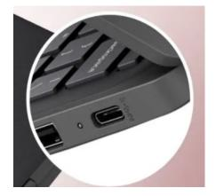
Instead, this new device has two USB-C connectors (one on either side) designed to replace all the other display standards outlined above.
